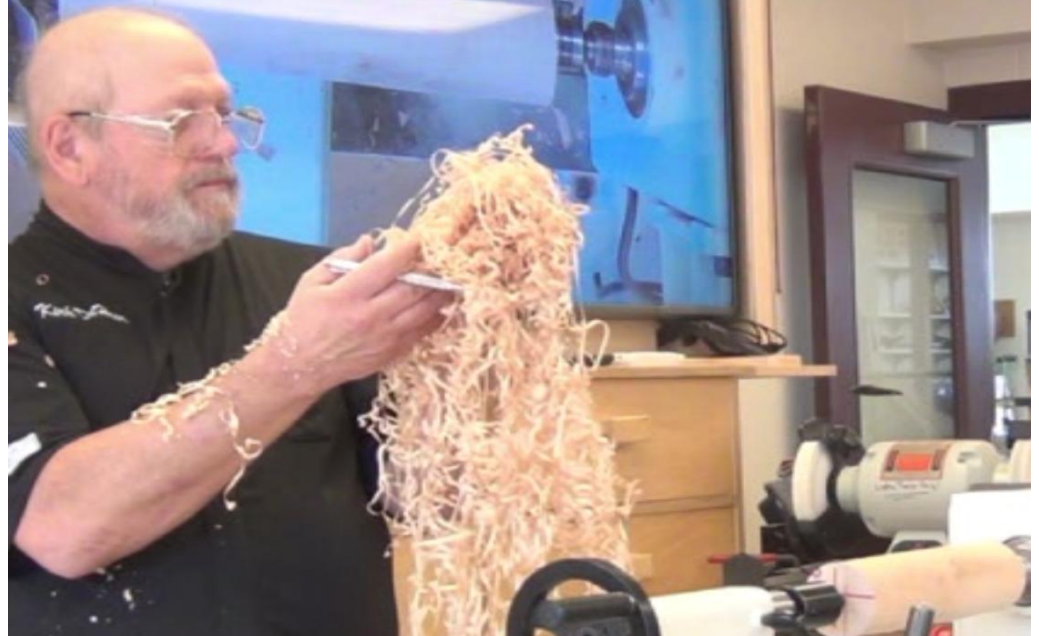
Properly cut shavings cut with a spindle roughing gouge after the blank is round
