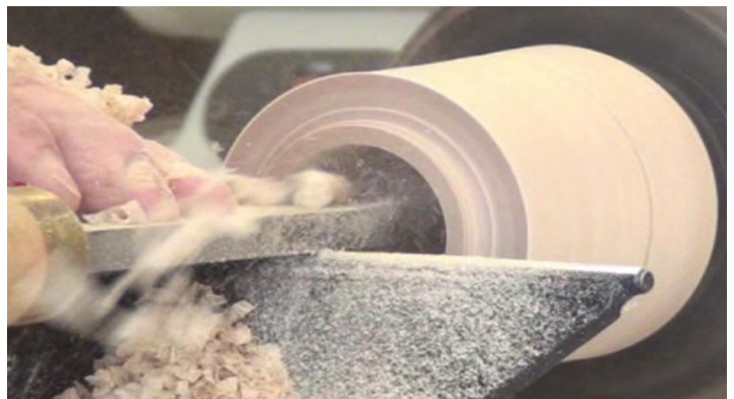
Hollowing the box. First he drilled a hole in the center with a spindle gouge. Then he rough hollowed the box cutting from the hole out to the wall. Last, he finished hollowing the box with a scraper.
