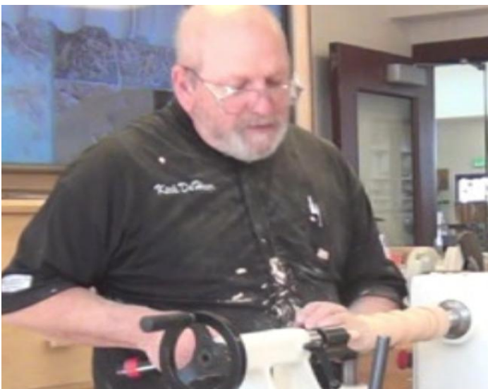
Cutting beads and coves with a spindle gouge
