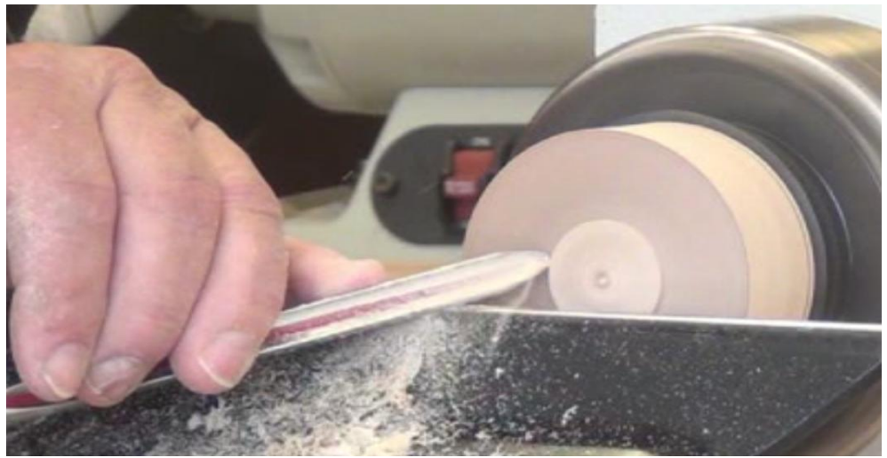
Turning end grain smooth and clean with a spindle gouge
