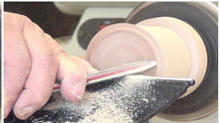
Finish cutting the bottom with the box on a jam chuck. Note the ring which lifts the box from the surface it sits upon.
