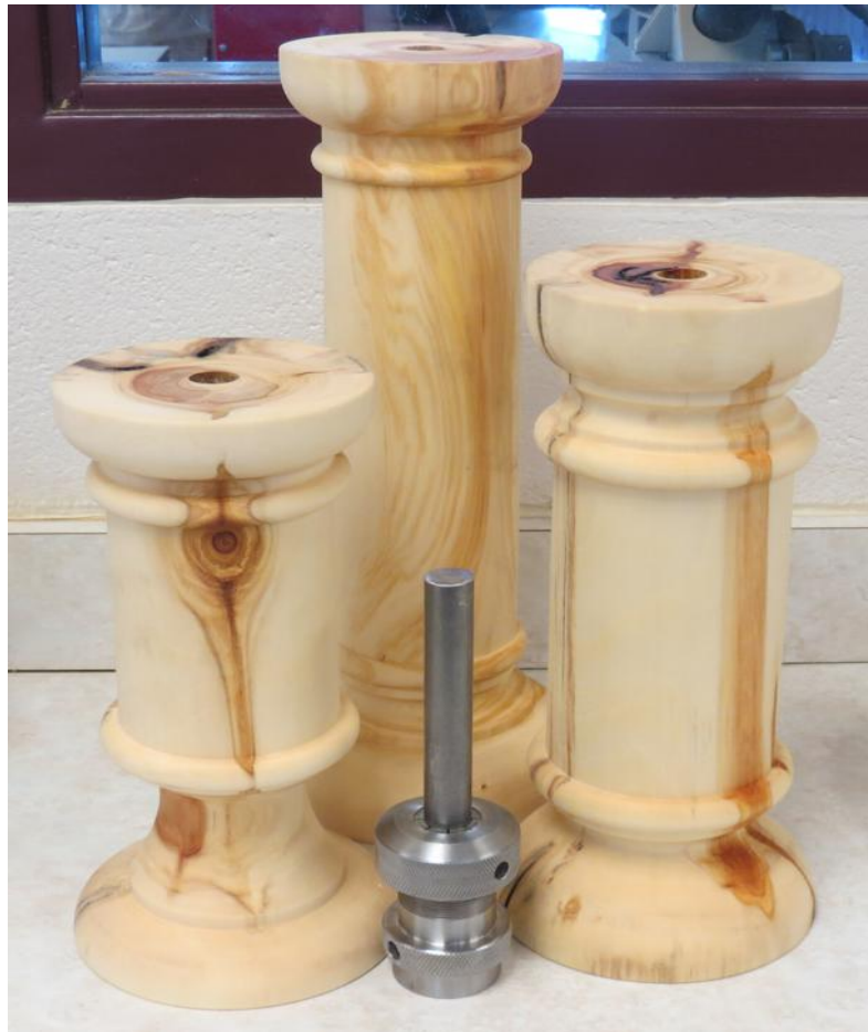
Leon Olson set of three large aspen candlesticks shown with the collet chuck and steel rod used to finish the bottom
