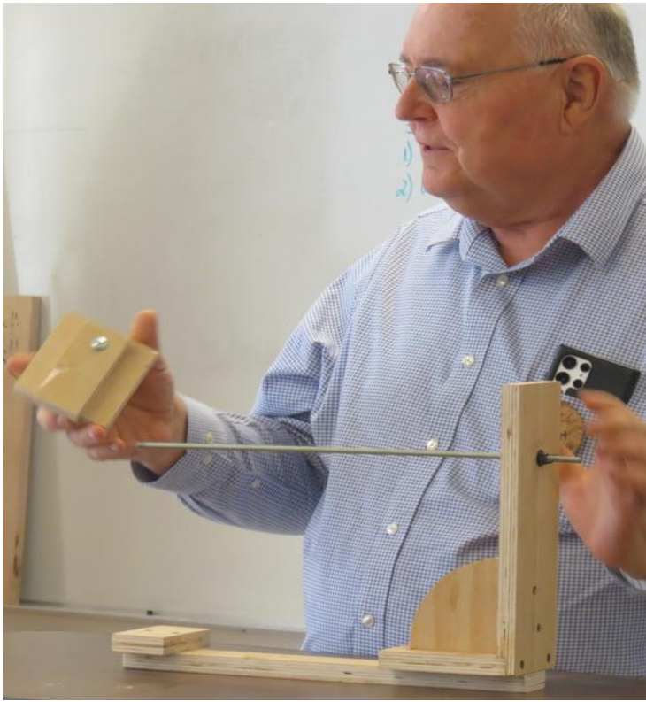
Karl McMullin brought in a device for measuring the thickness of the bottom of a bowl as he is turning.
