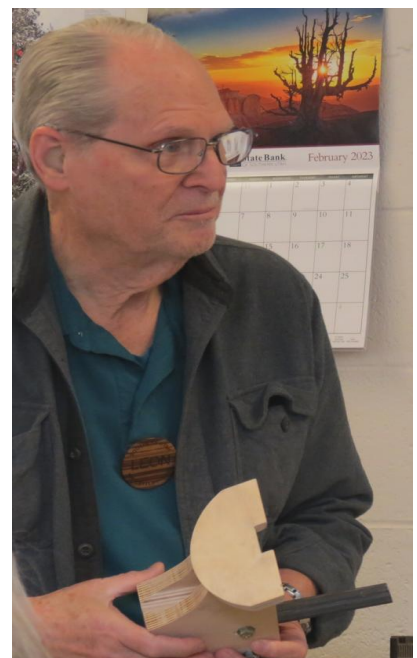
Leon Olson: Shop made grinding platform for Wolverine sharpening system
