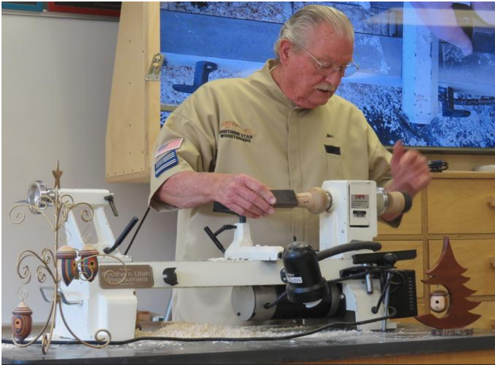
Jim with an expanding mandrel for holding the bird house blank on the lathe with another expanding mandrel for holding the roof in his hand. Mounting the bird house blank and turning it to shape. There is another mandrel for drilling the opening and the hole for a landing perch made with a round tooth pick.
