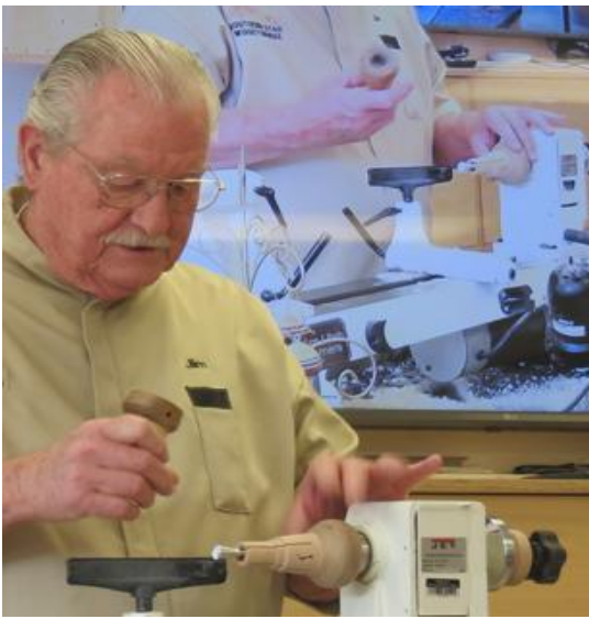
Jim with an expanding mandrel for holding the bird house blank on the lathe with another expanding mandrel for holding the roof in his hand. Mounting the bird house blank and turning it to shape. There is another mandrel for drilling the opening and the hole for a landing perch made with a round tooth pick.
