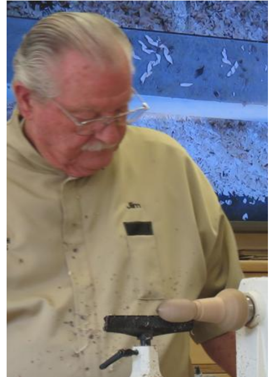
Jim with an expanding mandrel for holding the bird house blank on the lathe with another expanding mandrel for holding the roof in his hand. Mounting the bird house blank and turning it to shape. There is another mandrel for drilling the opening and the hole for a landing perch made with a round tooth pick.
